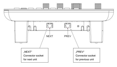
The cable specification has to match the EIA/TIA 568 B standard (shielded CAT5 with RJ45, AWG26).
