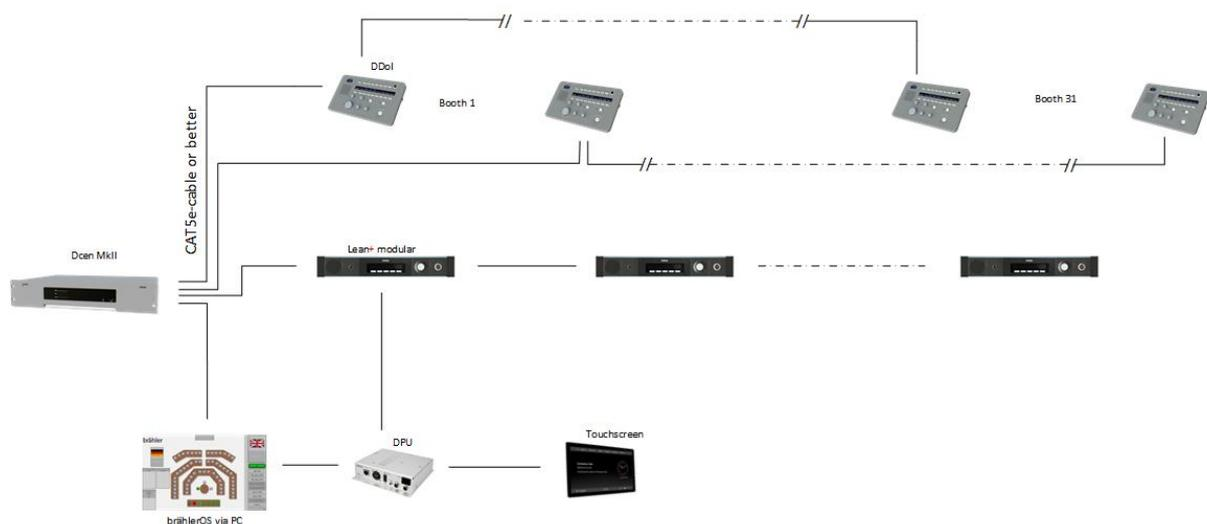
In this example application, DIGIMIC multimedia units SMic123W and SMic133D are connected to the DCen MkII. These allow, for example, viewing of documents relevant to the meeting. Votes, for example, are made via the touchscreen display.
