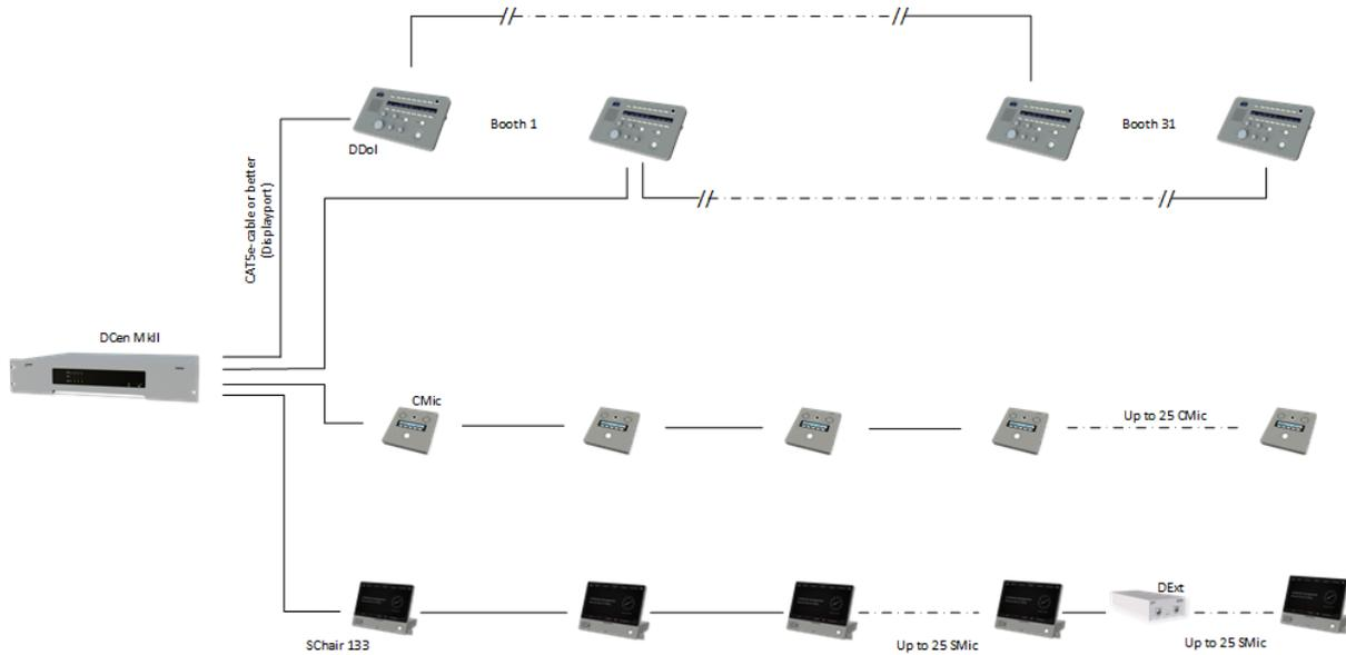
In the following system example, a DLine is interconnected in an SMic chain. This allows external audio signals (e.g. lectern) to be integrated into the DIGIMIC system and controlled like a microphone console.
