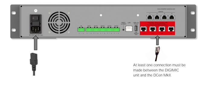
Now connect the individual elements that you need for your conference. All DIGIMIC components are connected to the central unit via the L1 - L4 sockets. Use suitable shielded CAT5e cables and RJ45 plugs.
