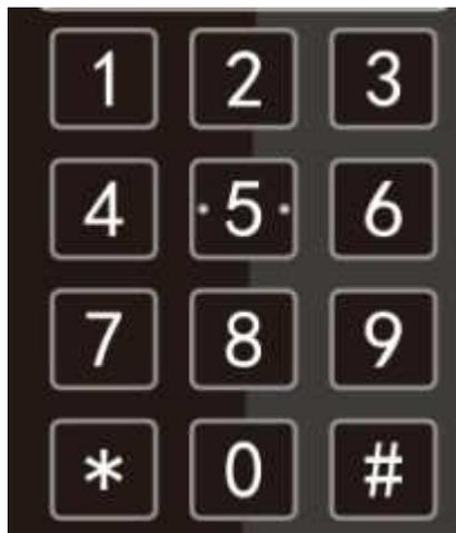
1. Preset setting: to set a preset position, the users should press the " 【SET PRESET】 " key first and then press the number key 0-9 to set a relative preset,
