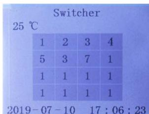
Switching an input to multiple outputs: press buttons "IN; 1" and buttons "OUT; 1; 2; 3; 4" (for example).
