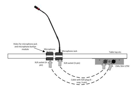
Now first connect CMic Slim UTM and microphone button and socket. Only use suitable cables.
