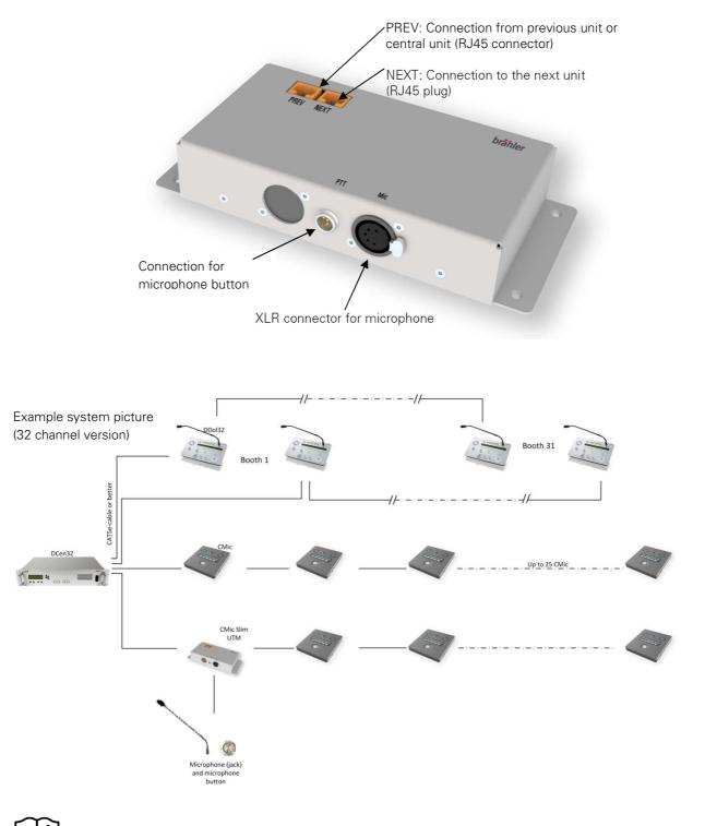
The CMic Slim UTM is not allowed to be connected in a chain with DIGIMIC interpreter units.
