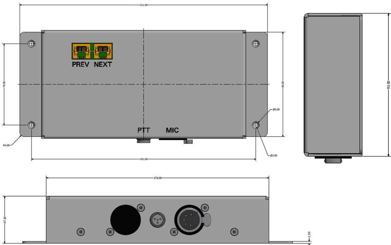
Drill holes in the destination of your microphone and microphone button. Fasten the appropriate modules (button and socket) in the drill holes (for drill sizes, please refer to the corresponding module). Attach the CMic Slim UTM to its destination (drill holes specified, see pictures above).
