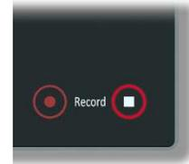
If the USB stick was not detected successfully, both buttons remain dark (no stick detected) or flash alternately (there is an error). In this case, use another USB stick or reformat the stick in FAT32 file format.
